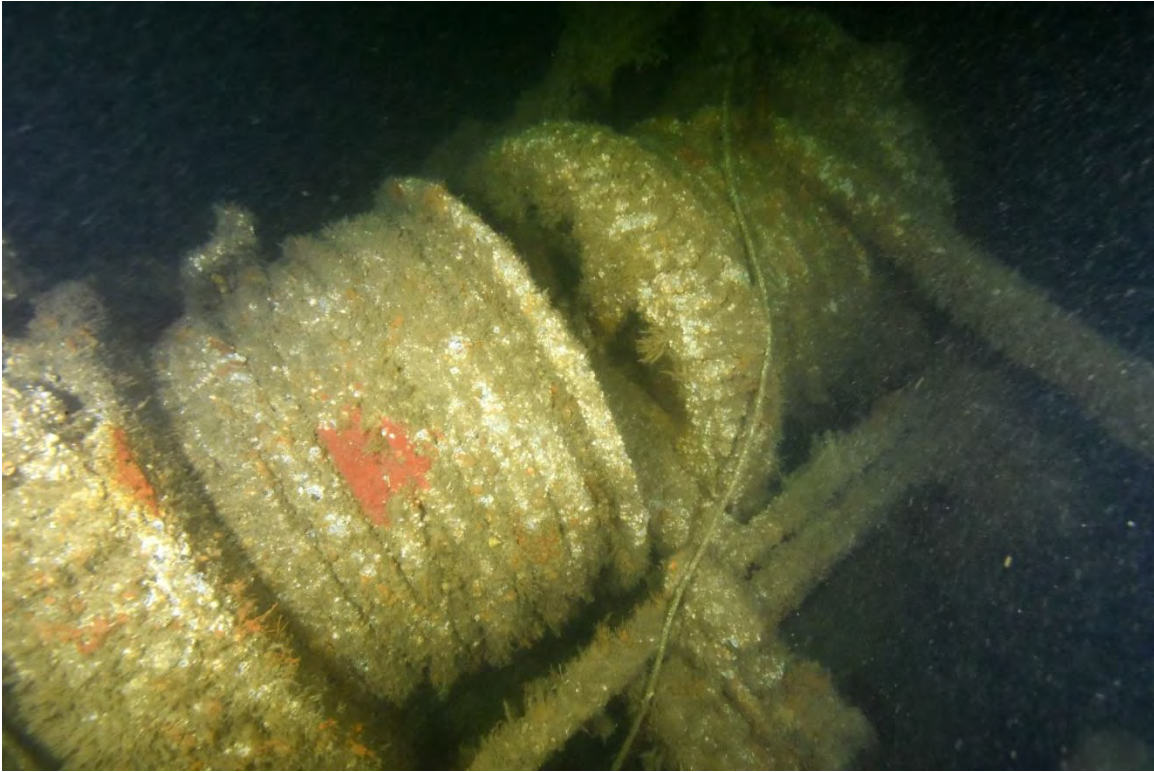
Figure 70 Heavy trawl winch used for minesweeping activity ©Martin Davies
