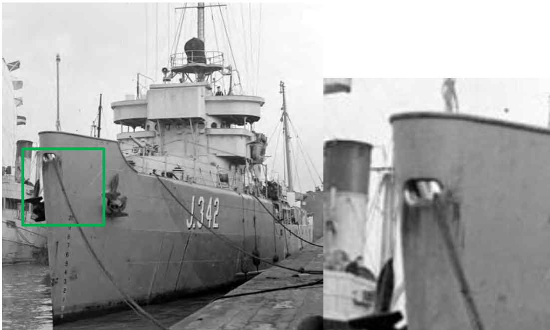
Figure 58 The Auk class 'Bullnose' - for mooring ropes.
