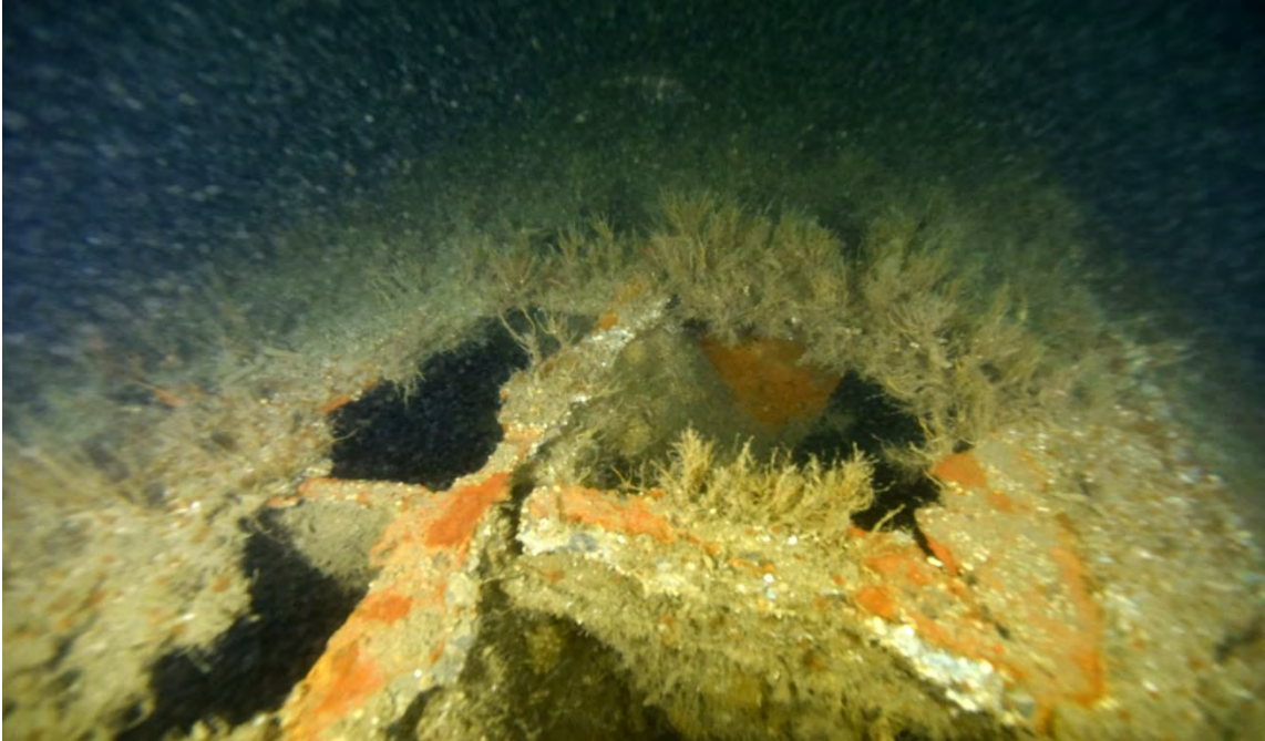
Figure 44. Numerous holes in the plating are visible along the length of the upturned hull ©Martin Davies
